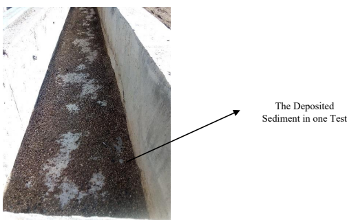
Figure 4. Deposited Sediments in the Channel in One Test to Determine the Weight of Deposition
