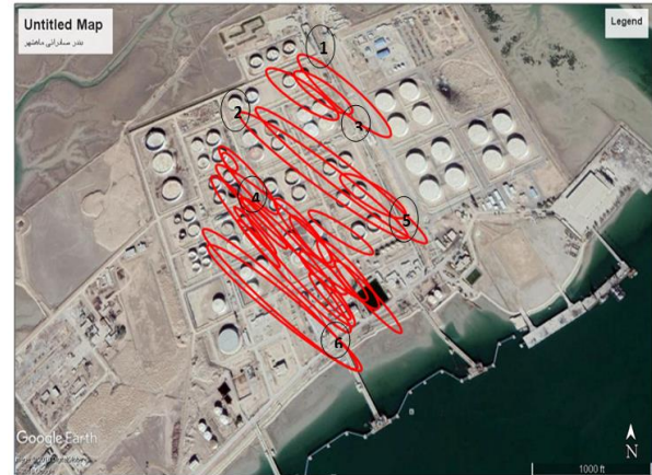
Fig. 3. VOC emissions from storage tanks in hot season and selected points for field measurements
