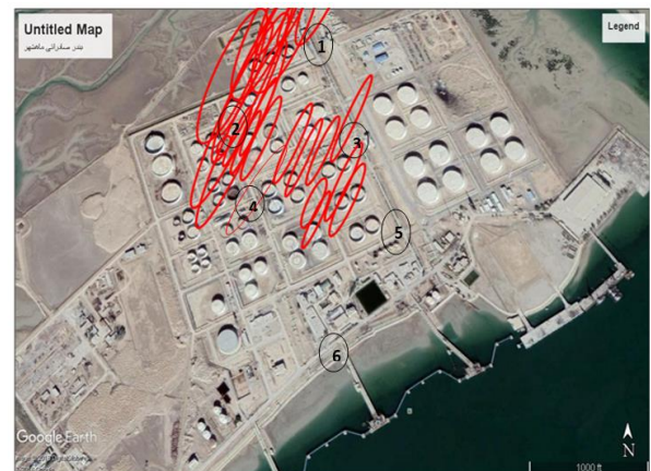
Fig. 4. VOC emissions from storage tanks in cold season and selected points for field measurements
