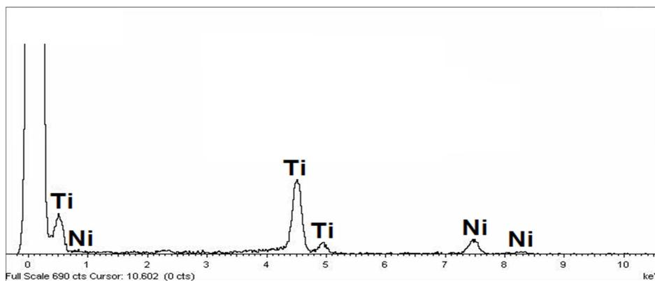
**Figure 4.** Energy dispersive X-ray (EDX) spectrometer patterns of dry titanium dioxide nanoparticles ( $nTiO_2$ ) powder [Ni signals in EDX spectrometer are from transmission electron microscopy (TEM) grid]
