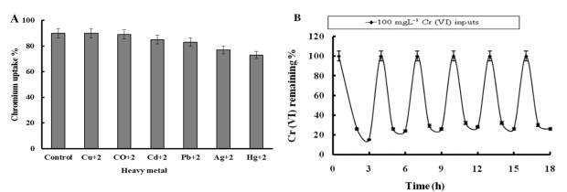
Fig. 2. (A) The effect of heavy metals on Cr(VI) reduction (%) by *Alcaligenes sp.* CKCr-6A, Error bars represent standard error. (B) Repeated detoxification of 100 mg/L Cr(VI) by CKCr-6A strain at 37°C in LB medium under 180 rpm of shaking without any amendment of nutrients
