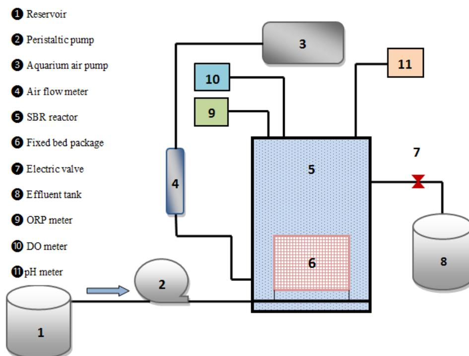
Figure 1. Schematic flow diagram of the experimental reactor
