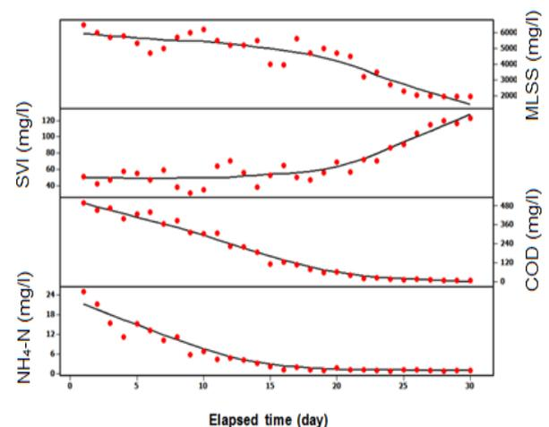
**Figure 2.** Variations in chemical oxygen demand (COD) and ammonium versus variations in sludge volume index (SVI) and mixed liquid suspended solid (MLSS) during acclimation period (Initial COD concentration = 500 mg/l, initial ammonium concentration = 25 mg NH<sub>4</sub>-N/l)
