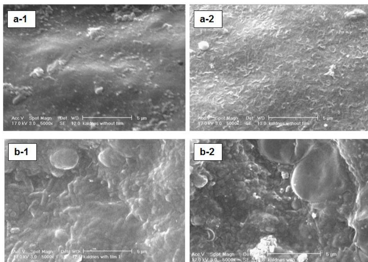
**Figure 3. Scanning electron microscopy (SEM) images of the (a-1) upper and (a-2) lower surface of the carrier without bio-film, (b-1) the carrier with bio-film and (b-2) the surface morphology of the bio-film after ammonium and chemical oxygen demand (COD) removal in saline wastewater taken at 5000 X magnification**
