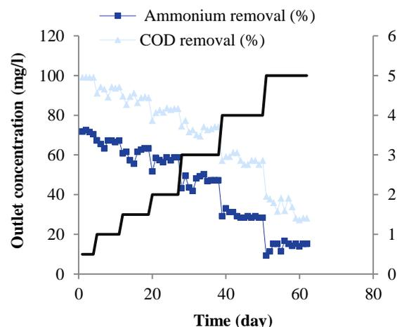
**Figure 6.** Effect of salinity on the removal percentage of ammonium and chemical oxygen demand (COD) during 62 days of operation (Initial COD concentration = 1000 mg/l, initial ammonium concentration = 50 mg  $\text{NH}_4\text{-N/l}$ )
