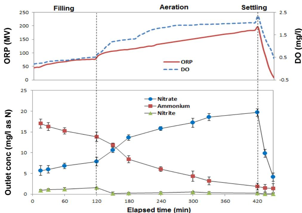
Figure 4. Variations in the nitrogen species concentration, and dissolved oxygen (DO) and oxidation-reduction potential (ORP) values versus elapsed time (Initial ammonium concentration = 25 mg NH<sub>4</sub>-N/l)
