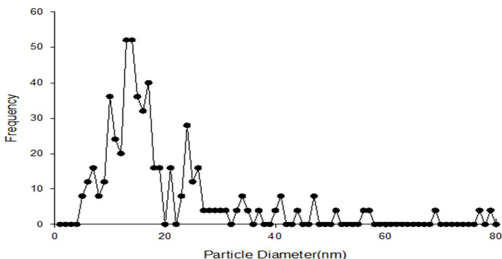
Figure 2. Size distribution of particles based on number frequency determined from transmission electron microscope data in dry titanium dioxide nanoparticles (nTiO<sub>2</sub>) powder
