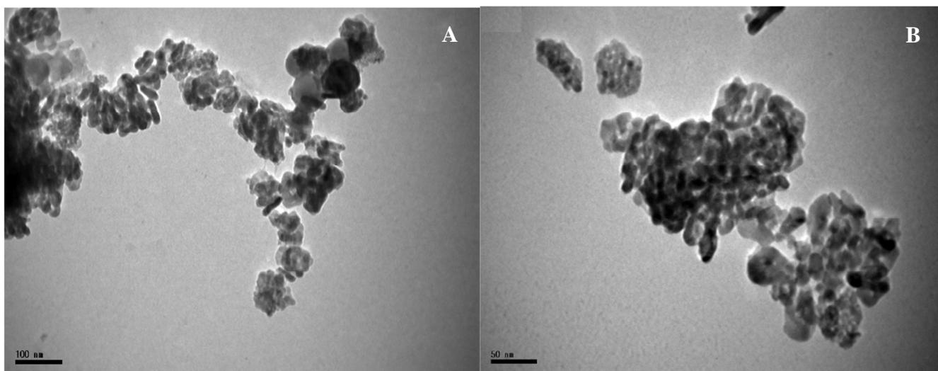
Figure 1. Transmission electron micrographs of dry titanium dioxide nanoparticles (nTiO<sub>2</sub>) powder (A) and aqueous suspension of nTiO<sub>2</sub> (B)
