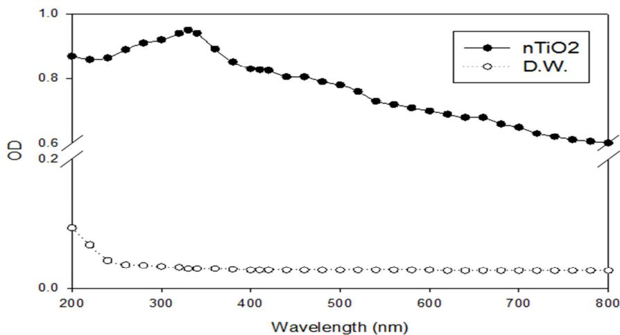
**Figure 5.** UV-VIS absorption spectra of suspensions of titanium dioxide nanoparticles (nTiO<sub>2</sub>) and distilled water (D.W.)
